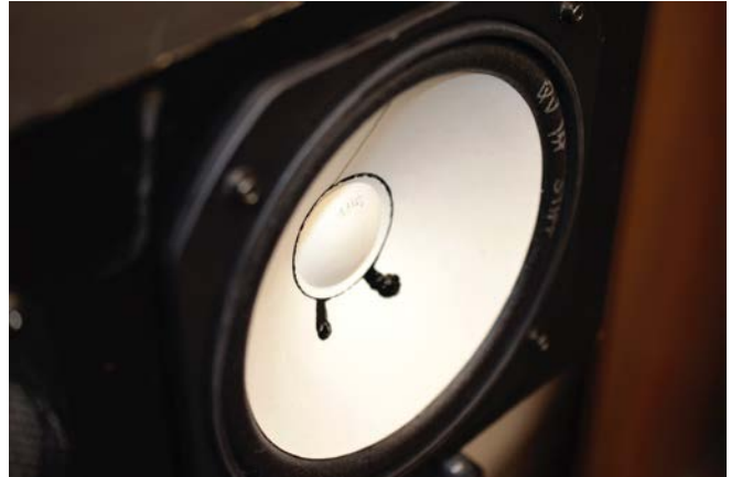
MS10-W prototype mounted in NS10M enclosure. Note the cone seam.
