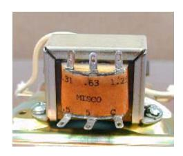
TAPS AT: COMMON 5 W ATT 2.5 W ATT 1.25 WATT .063 WATT .031 WATT
